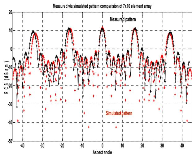
Figure 1. RCS versus aspect angle comparison of simulation and measurement of fiber array (7 x 10) at 3 GHz
