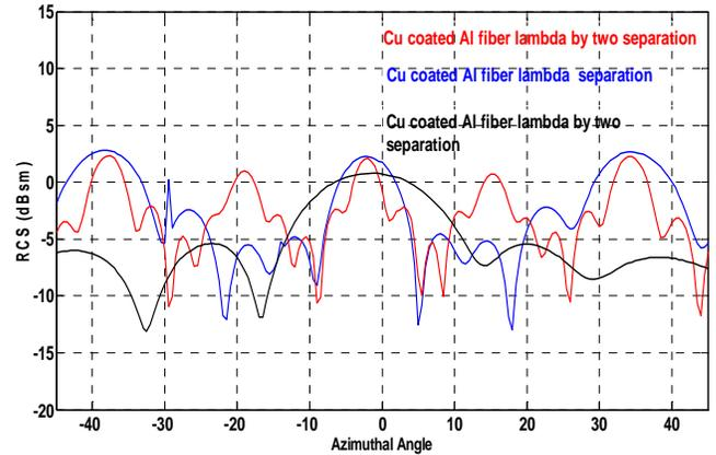
Figure 10. RCS versus azimuth angle comparison of Aluminum coated glass fiber array with  $2\lambda$ ,  $\lambda$  and  $\lambda/2$  separation at 4 GHz
