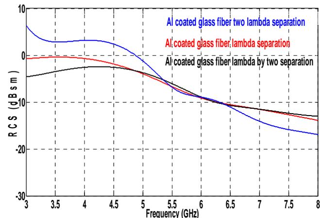
Figure 6. RCS versus frequency comparison Aluminum coated glass fiber array (8x5) with  $2\lambda$  ,  $\lambda$  and  $\lambda/2$  separation
