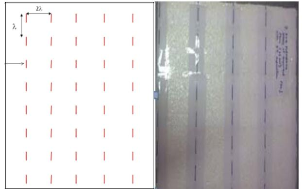
Figure 2. Linear distribution with  $2\lambda$  separation line by line and  $\lambda$  separation collinear (Schematic and prepared sample).
