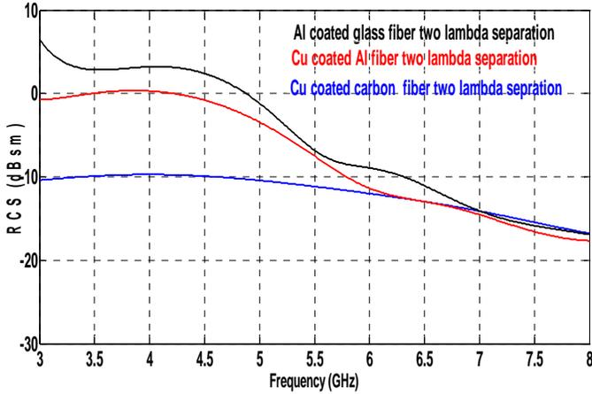
Figure 7. RCS v/s frequency comparison Aluminum coated glass fiber , copper coated carbon fiber and copper coated Aluminum fiber (8x5).
