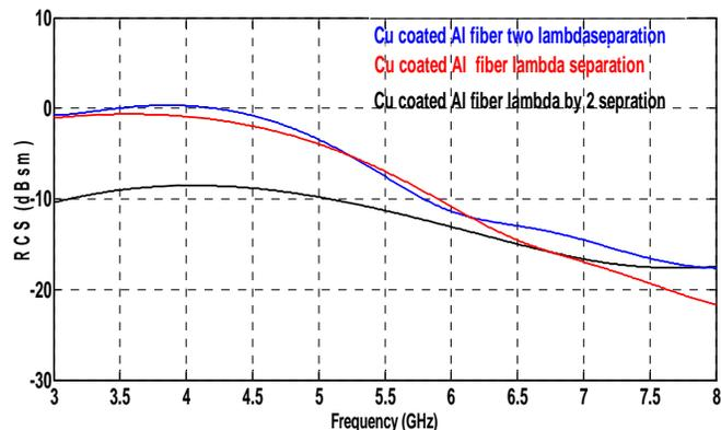
Figure4. RCS versus frequency comparison of copper coated Aluminum fiber array (8x5) with  $2\lambda$  ,  $\lambda$  and  $\lambda/2$  separation
