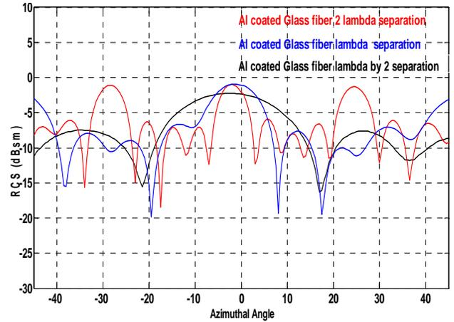
Figure 9. RCS versus azimuth angle comparison of Aluminum coated glass fiber array with  $2\lambda$ ,  $\lambda$  and  $\lambda/2$  separation at 5GHz
