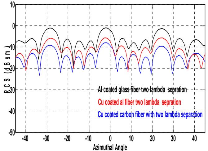
Figure 11. RCS versus azimuth angle comparison of Aluminum coated glass fiber, copper coated carbon fiber and copper coated Aluminum fiber at 5GHz
