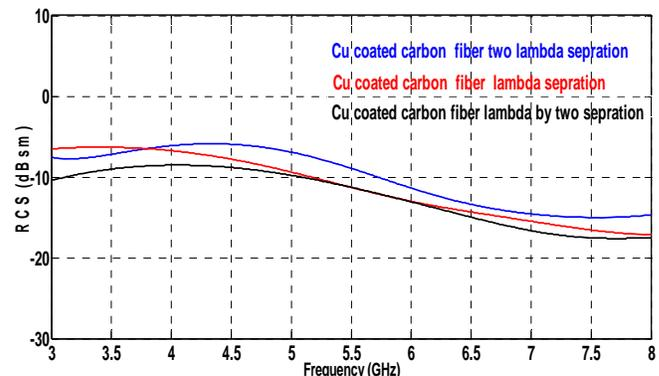
Figure 5. RCS versus frequency comparison of copper coated carbon fiber array with  $2\lambda$  ,  $\lambda$  and  $\lambda/2$  separation
