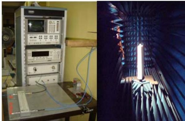
Figure 3 VNA Instrumentation and Anechoic Chamber for RCS
