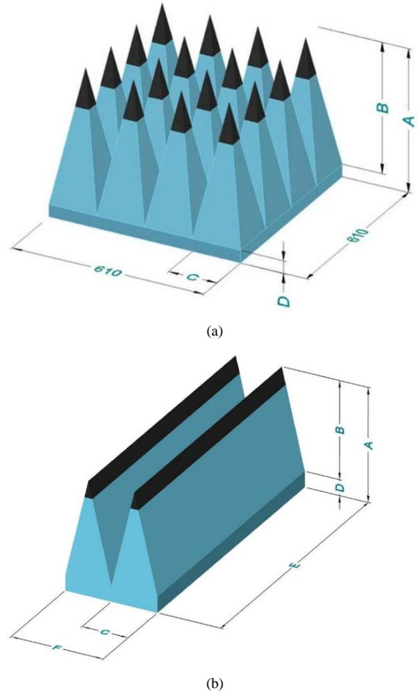
Fig. 1. Schematic view of the 2 main wideband absorbers used to line the walls of an anechoic chamber; (a) Pyramidal Absorber. (b) Wedge absorber.
