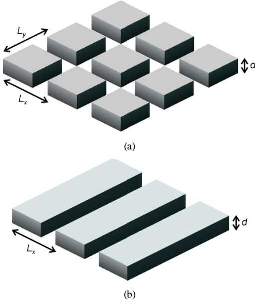
Fig. 2. Schematic illustration of the basic layers forming the two considered absorbers; (a) Pyramidal Absorber. (b) Wedge absorber.
