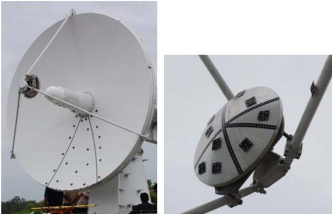
Figure:-1 Ground Station Antenna Measurements using CRP
